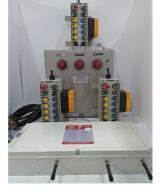
In the month of April 2017, Speed-O-Controls Pvt. Ltd. designed and supplied a special Radio Remote application to their long term client Electrosteel. The client had requested for Wall mounted Remote systems due to limited access of the floor shop. The most critical criteria was to ensure that the range of the radio frequency does not get affected. SOC designed a special Radio module for these Wall Mounted Systems. The systems have been supplied and are working satisfactorily
